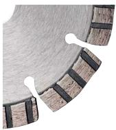
Depending on the type, the segments are laser welded or sintered onto the body. As is well known, diamonds are one of the hardest materials around and they do the actual work when cutting or drilling.
